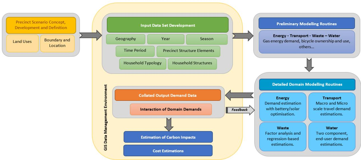
Figure 2 ETWW operational flowchart
