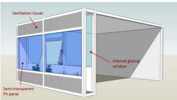
Figure 1: Sample effect picture of the BIPV/T-DSF system in the building.
