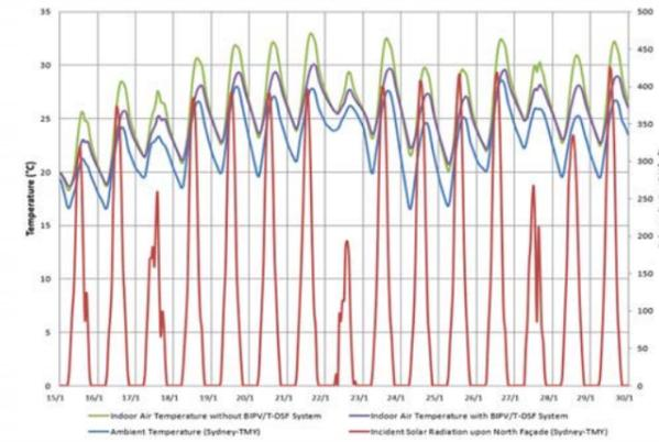
Figure 3: Indoor air temperature with/without BIPV/T-DSF in summer.
