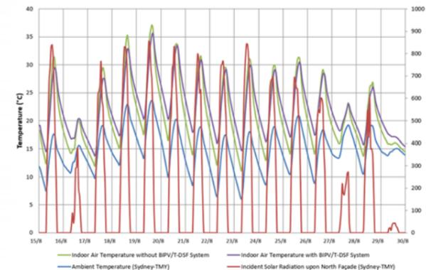
Figure 4: Indoor air temperature with/without BIPV/T-DSF in winter.
