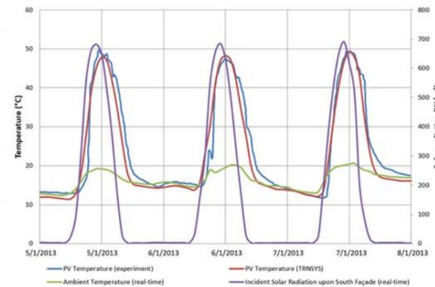
Figure 2: Validation of PV module temperature under buoyancy-driven ventilation (MBE = 4.55%; CVRMSE = 14.48%).
