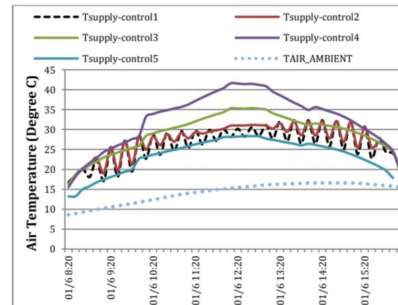
The integration of this BIPV/T model into various residential buildings was investigated using TRNSYS software. It was determined that the best suitable house for the integration of this system is a well-insulated building with heavy mass constructions and double glazed windows, shaded externally in temperate climates. Figure 4 shows the indoor air temperature of a potential house with/without BIPV/T systems in Sydney.
