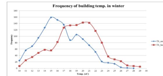
Figure 5: Frequency of building temperature in winter (hourly, 1 degree bins).
