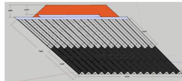
Figure 2: Top-down view of the PV/T and Solar Thermal System Design.
