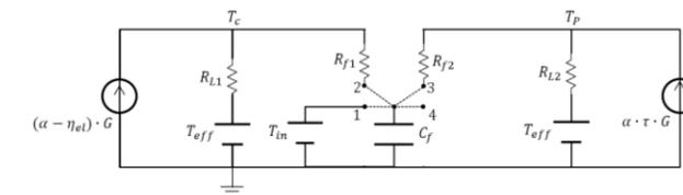
Figure 3: Equivalent thermal circuit of the PV/T and solar thermal air collectors established for the detailed analysis.
