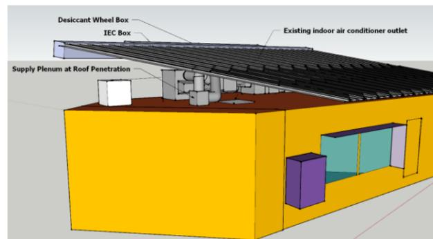
Figure 1: Final design of the PV/T desiccant wheel cooling system
