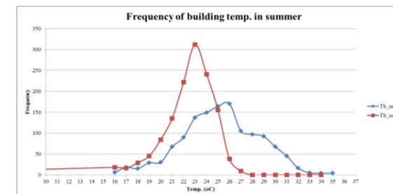
Figure 6: Frequency of building temperature in summer (hourly, 1 degree bins).
