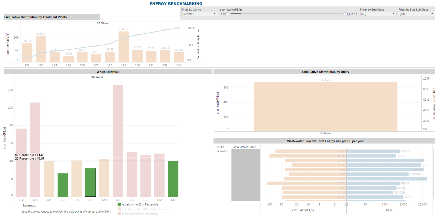
Figure 3 Layout of (beta version) Benchmarking Energy and Carbon (BEC) tool Tableau dashboard.
