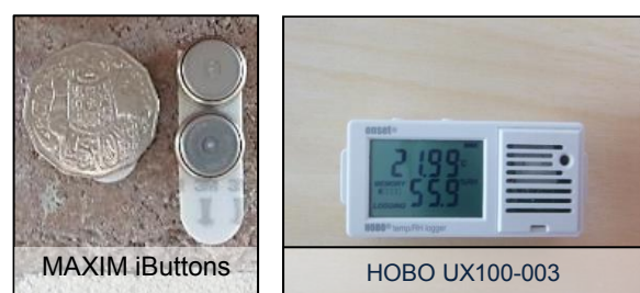
Figure 2. HOBO and iButton temperature and relative humidity loggers employed in the current study
