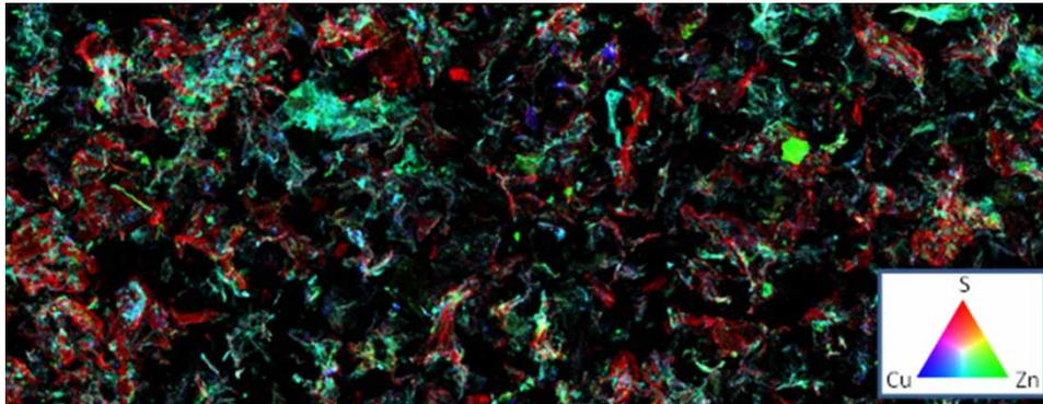
**Figure 5** | Tricolor map from the X-ray fluorescence microscopy of AGS showing sulfur (red), zinc (green) and copper (blue). The full colour version of this figure is available online at <http://www.iwaponline.com/wst/toc.htm>.
