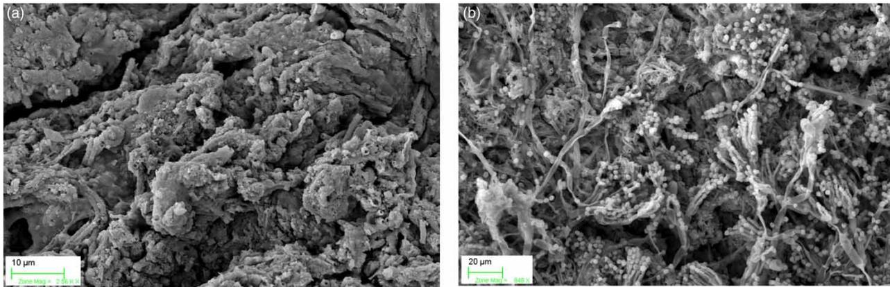
**Figure 4** | Scanning electron micrographs comparing the surface structure of (a) AGS granules taken from Strategy B (33% anaerobic feed) and (b) biomass from strategy C (100% aerobic feed). Scale bar represents 10 μm and 20 μm respectively.
