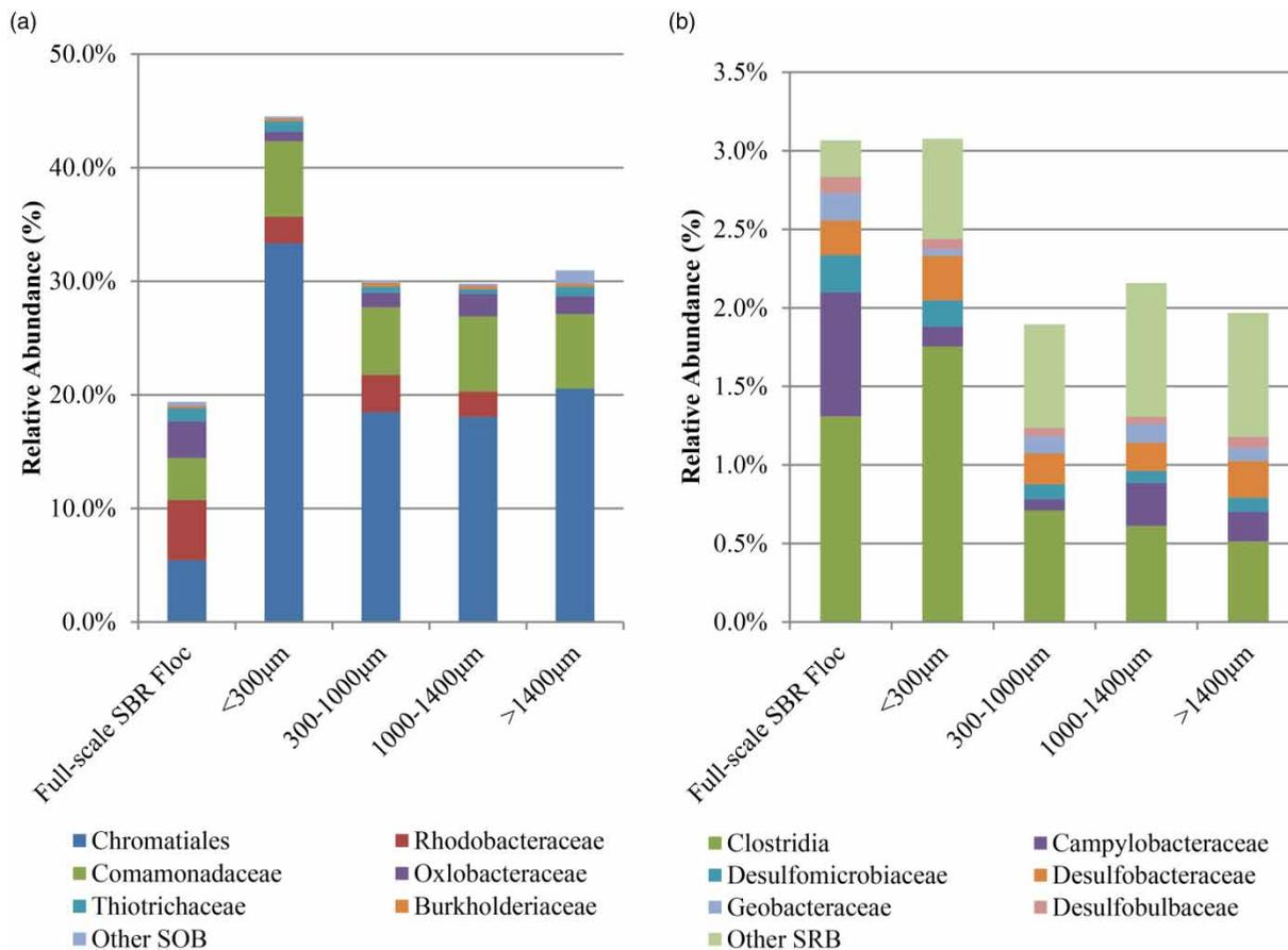
**Figure 3** | Changes in abundance of sulfide-oxidising bacteria (a) and sulfate-reducing bacteria (b) of size-separated granules (<300, 300–1,000, 1,000–1,400 and >1,400 µm) that were sampled during Strategy B (33% anaerobic feed), with comparison to Strategy C (full-scale 100% aerobic feed).
